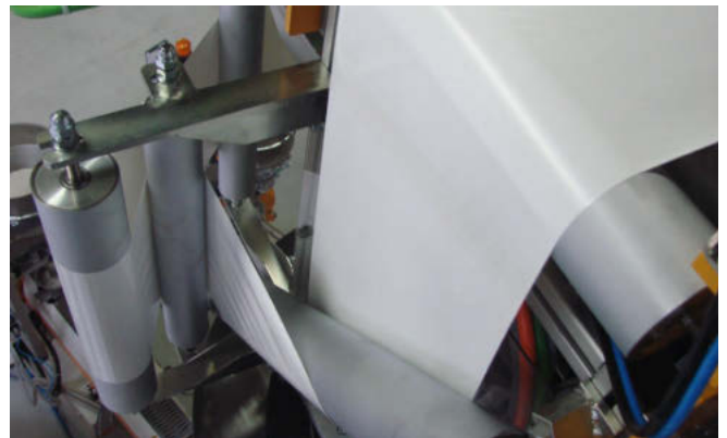
Perfect, precision-wound film rolls thanks to turning-bar haul-off.
